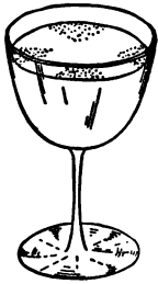
FIG. 73. A wine glass filled with water vibrates when a fiddle bow is drawn across its edge. Touch the glass lightly with your finger and notice that at four places there are no waves. (Try it.)
